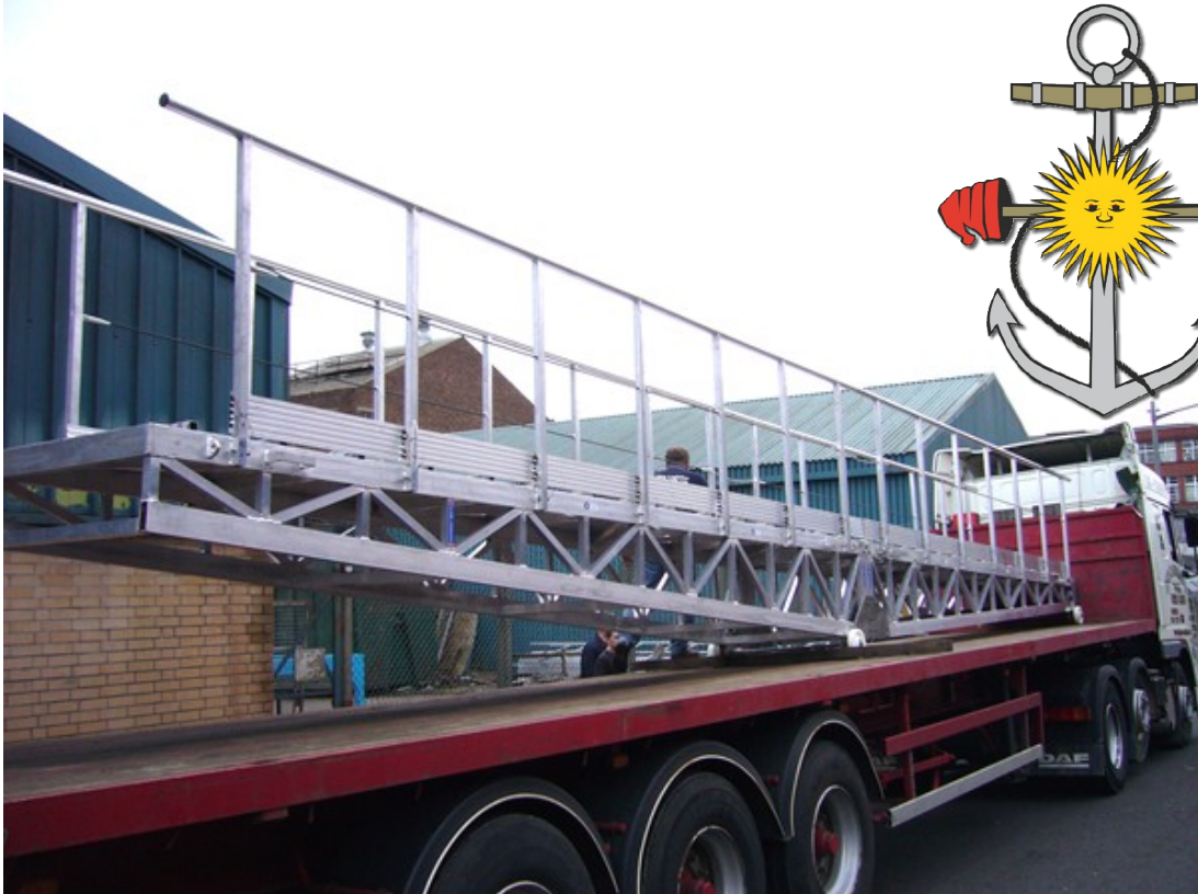
An angled gangway, designed to pivot on a central point, built for the Argentine Navy.
